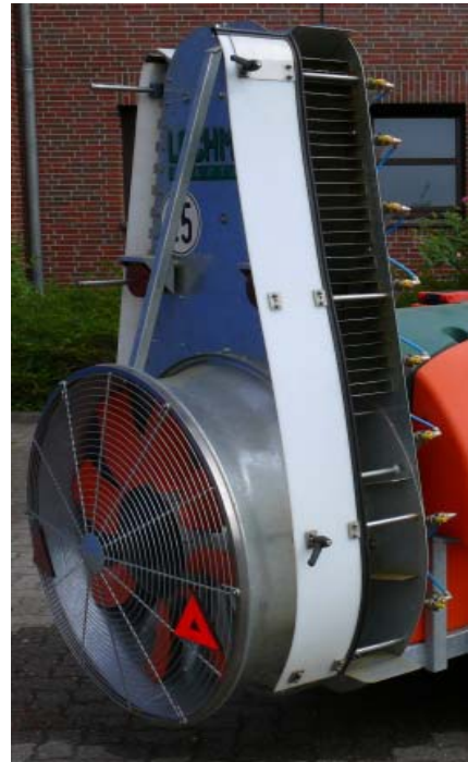
Fig.8: Axial fan „90 Q“ with 900 mm rotor
