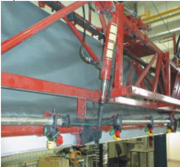
Figure 2: Spray boom with air conduction via synthetic fabric hoses and outlets which are adjustable as to direction.
