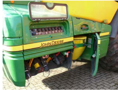
Fig.8: Control centre and induction hopper on right sprayer side.
