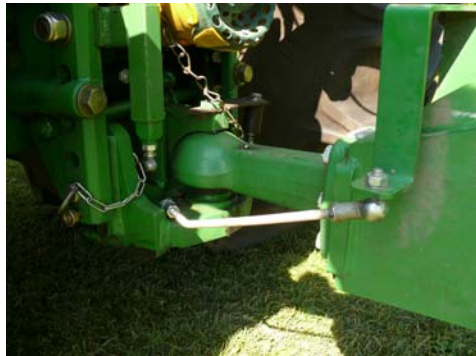
Fig.5: Draw bar with steering sensor.
