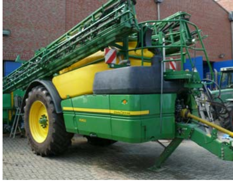
Fig.4: Sprayer with lateral folded boom.
