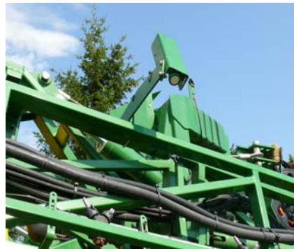
Fig.7:Folded boom with BoomTrac sensor.
