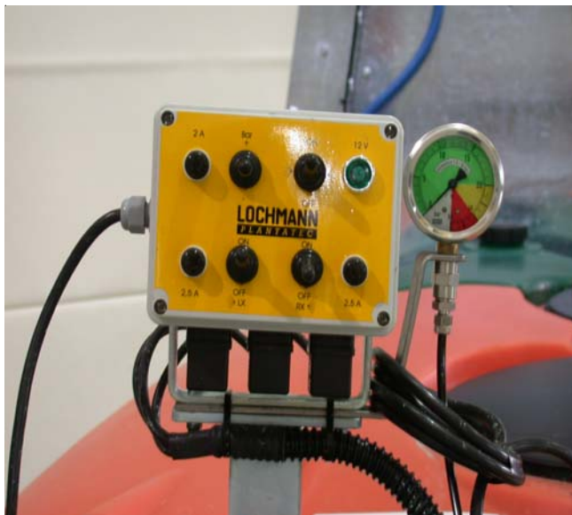
Fig.5: Manually operated control valves
