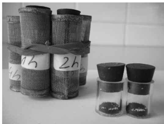
Figure 2 Small glass tubes for exposure of drugstore beetle eggs, and egg cages enclosed into wire mesh cages for testing.
