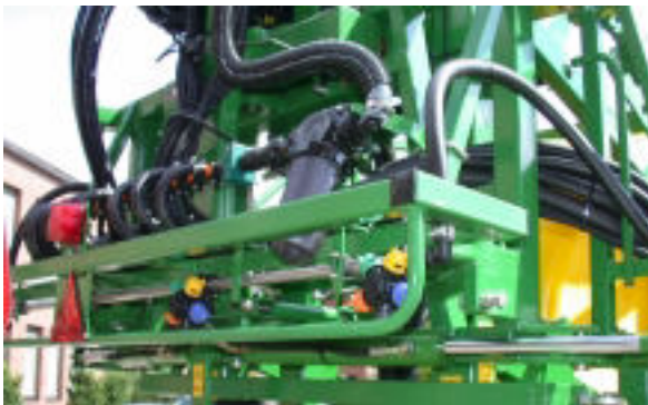
Figure 7: VRS-return flow pipes with collective breeching and filter at the spray boom.
