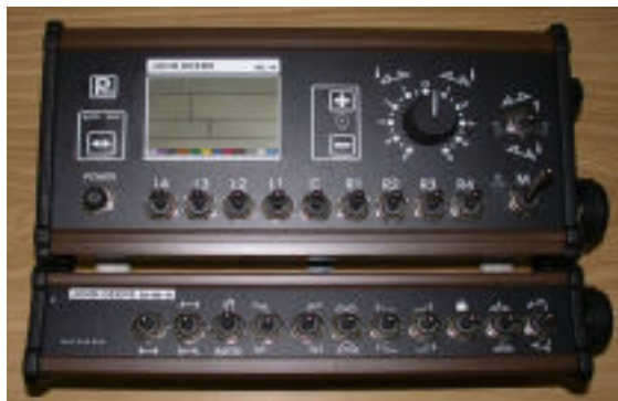
Figure 6: Operator control panel EL - 4.
