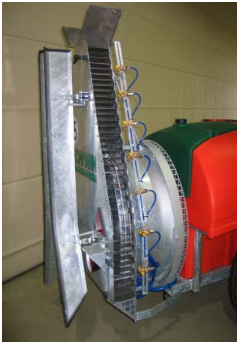
Fig.7: Axial fan „80 UQ“ with 800 mm rotor and air intake at the front
