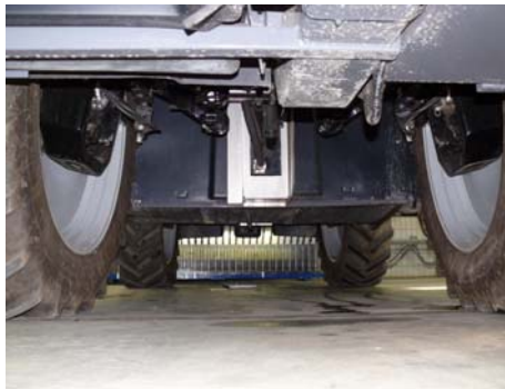
Fig.5: The smooth floor pan with up to 1.16 m ground clearance.
