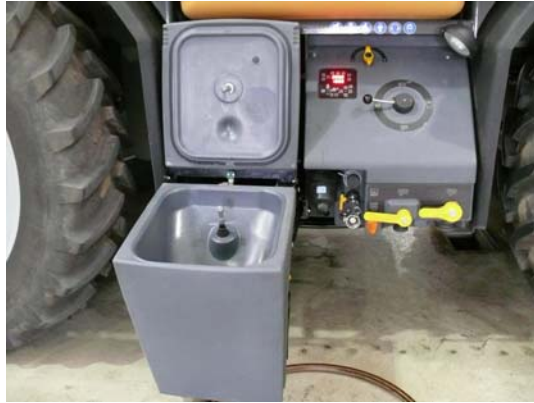
Fig.6: Left sprayer side with control panel and induction hopper.
