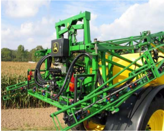
Fig.5: boom suspension with control valves.
