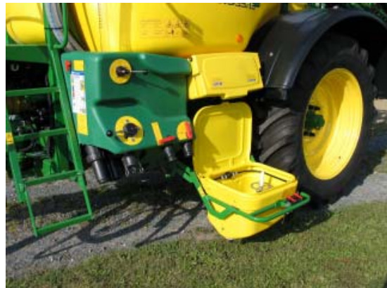
Fig.9: central controls on the left side of the sprayer and easily accessible induction bowl.
