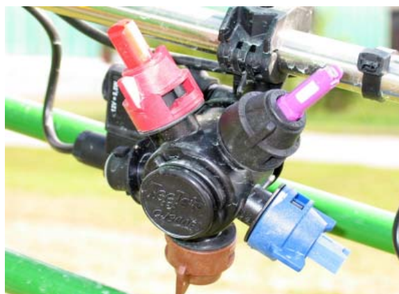
Fig.4: multi-nozzle body on the boom pipe.
