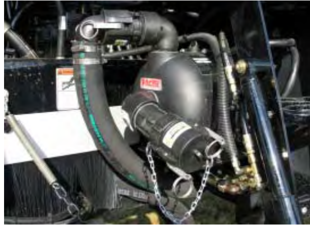
Fig. 6: Filling pump with Kamlock - connection.
