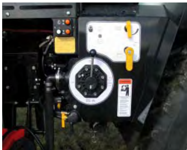
Fig.7: Central controls at the left hand side with buttons (orange) for adjusting the engine revolutions.
