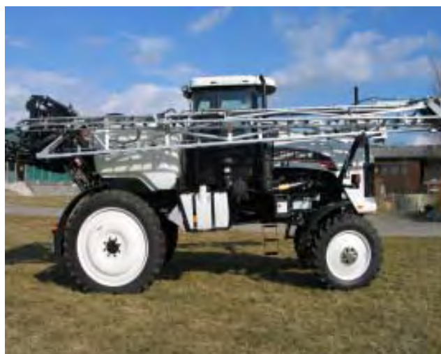
Fig.4: Right sprayer side. You see the rinsing water tank in front of the rear wheel.
