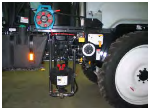
Fig. 9: Left sprayer side with induction hopper in working position (in the centre) and tube for outer surface cleaning.
