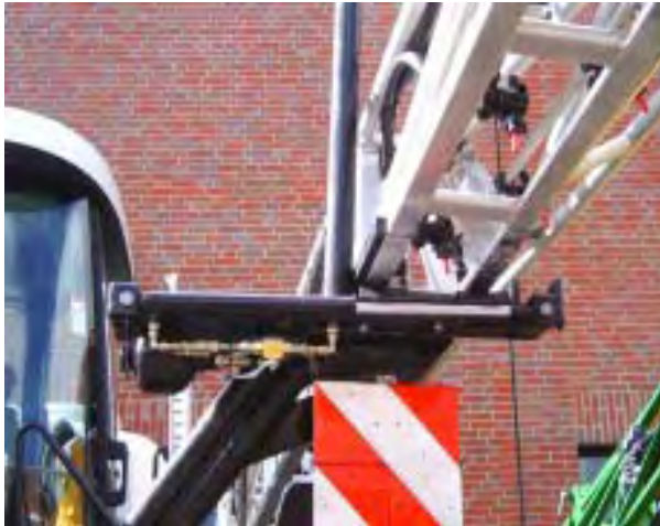
Fig. 8: Moveble boomrest for easier entry of the cabin.
