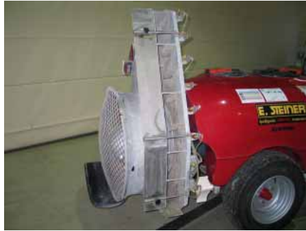
Fig.6: Axial fan with 800 mm rotor
